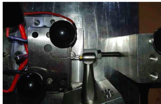
motor (Silver Reciproc, VDW) at 400 rpm in continuous rotation as recommended by the manufacturer. Torque was set at the maximum value. Each instrument was positioned in the contra-angle handpiece and introduced into the canal at the same position (16 mm). To reduce the friction of the file as it touched the artificial canal walls, a special high-flow synthetic oil designed for lubrication of mechanical parts (Super Oil; Singer Co Ltd, Elizabethport, NJ) was applied.
