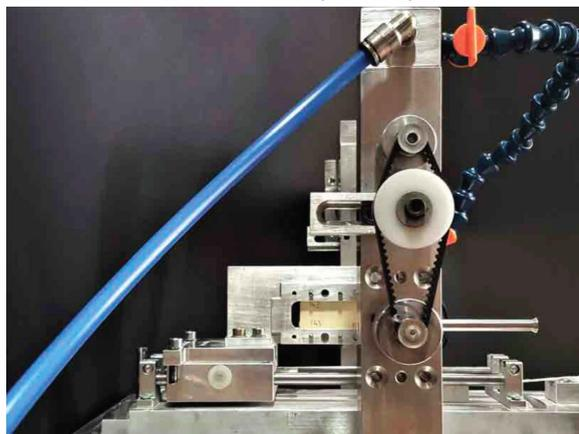
Figure 1. Customized testing machine employed for cutting efficiency tests.
